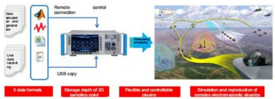
Fig. 1.7 Downloading and Playing of Arbitrary Waveform Data
