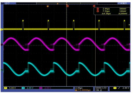
Fig.3.24 Diagram of Arbitrary Trigger (Continue/Realtime)
