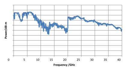
Fig. 1.3 Max. Output Power of S1465F+H05
