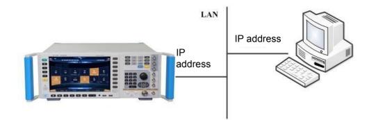
Fig.5.4 LAN Interface Connection
