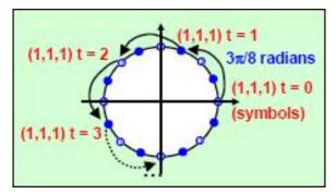
Attached Figure 10 EDGE Vector Diagram
