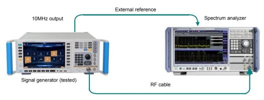
Fig.7.6 Low Power Test
