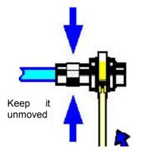
Fig.2.6 Completion of Final Connection with a Torque Wrench
