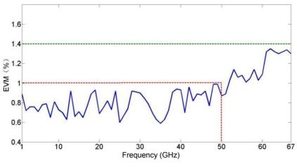
Fig. 1.8 Vector Modulation Accuracy
