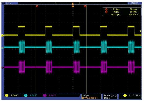
Fig.3.22 Diagram of Baseband Triggering (Gate/High)
