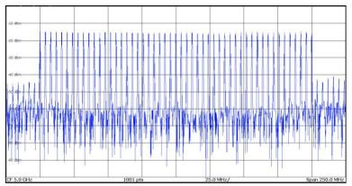
Fig. 1.5 5GHz Carrier 200MHz Modulation Bandwidth Multi-tone Signal
