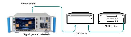
Fig.7.3 Internal Time Base Aging Rate Test
