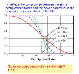
Attached Figure 11 Diagram of Relation between Channel Bandwidth and  $\alpha$
