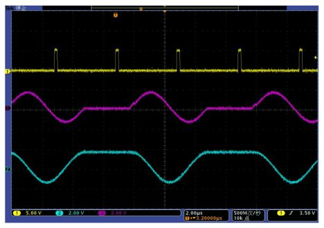
Fig.3.25 Diagram of Arbitrary Trigger (Single/Ignore Repeated Trig)
