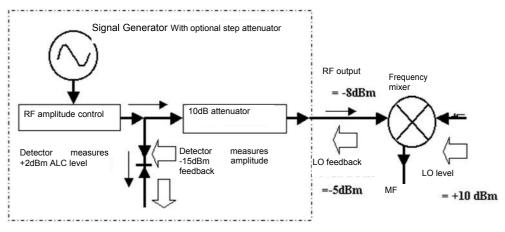
Fig.3.12 Effects of Reverse Power (-8dBm Non-coupling Output)
