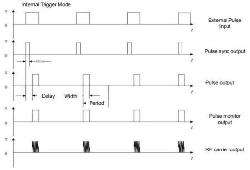
Fig.3.17 Internal Trigger Mode
