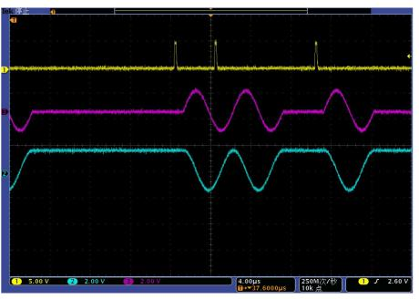
Fig.3.26 Diagram of Arbitrary Trigger (Single/Buffer Repeated Trig)
