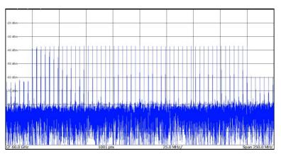
Fig. 1.6 60GHz Carrier 200MHz Modulation Bandwidth Multi-tone Signal
