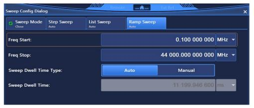
Fig.3.7 Ramp Sweep configuration dialog
