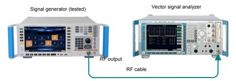
Fig.7.9 EVM and Original Offset Test
