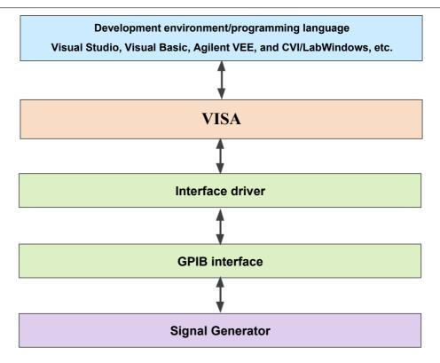
Fig.5.6 Programmable Software and Hardware Layers
