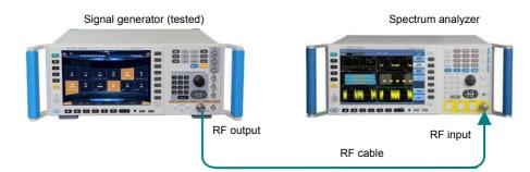
Fig.7.8 Pulse Modulation Rise/Fall Test
