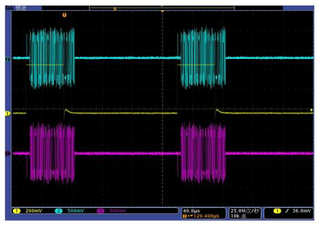
Fig.3.21 Diagram of Baseband Triggering (Continues/Single)
