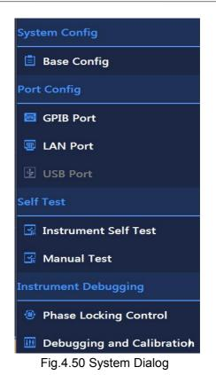
System Dialog, shown in Fig.4.50, enables you to set four main modules: System Config, Port Config, Self Test and Instrument Self Test.
