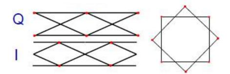
Attached Figure 8 QPSK Modulation Method
