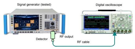
Fig.7.7 Pulse Modulation On-off Ratio Test
