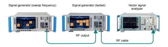
Fig.7.10 External FM Frequency Response Test
