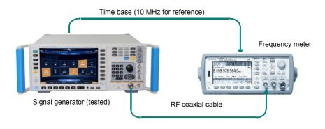
Fig.7.2 Frequency Resolution Test
