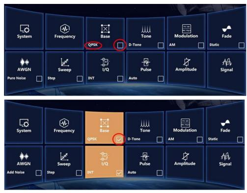
Fig.2.15 Shortcut Operations Schematic
