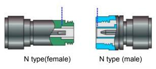
Fig.2.8 Calibration Surface
