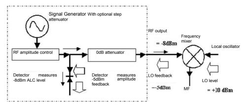
Fig.3.11 Effects of Reverse Power (-8dBm Coupling Output)
