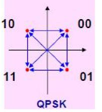
Attached Fig.2 QPSK Diagram
