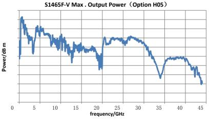
Fig. 1.4 Max. Output Power of S1465F-V+H05
