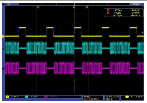
Fig.3.23 Diagram of Baseband Triggering (Gate/Low)
