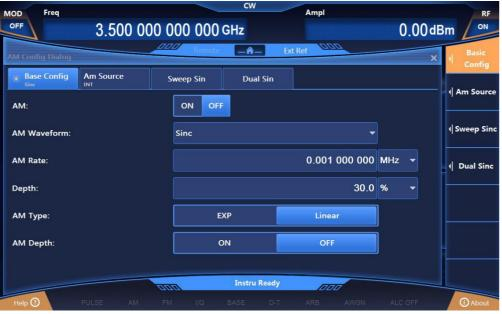
Fig.2.22 Setting of Amplitude-modulated Signals
