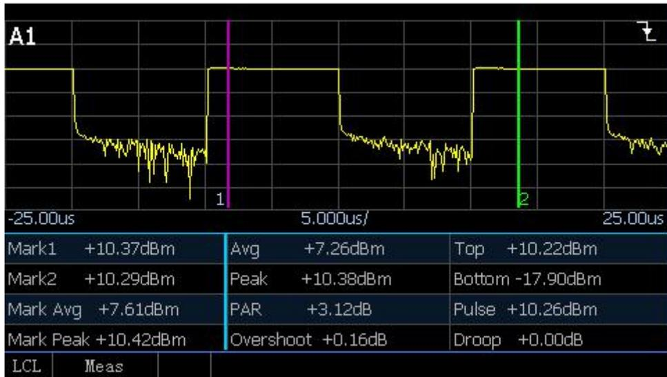
Fig. 3.2 Automatic measurement of power parameters in several periods
