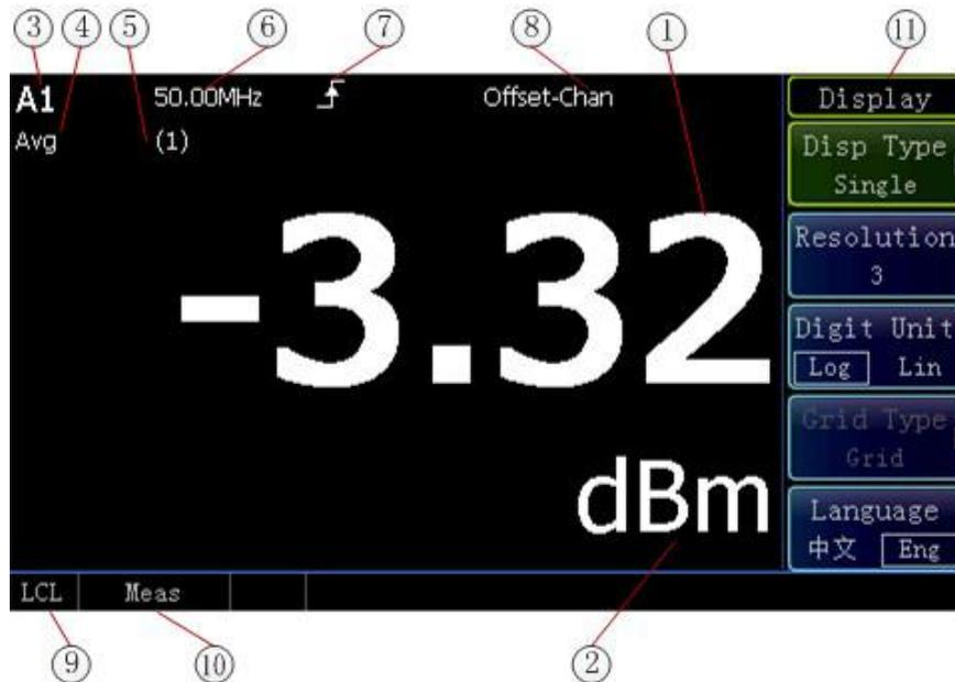
Fig.2.11 Measurement interface in case of connection with a peak power sensor
