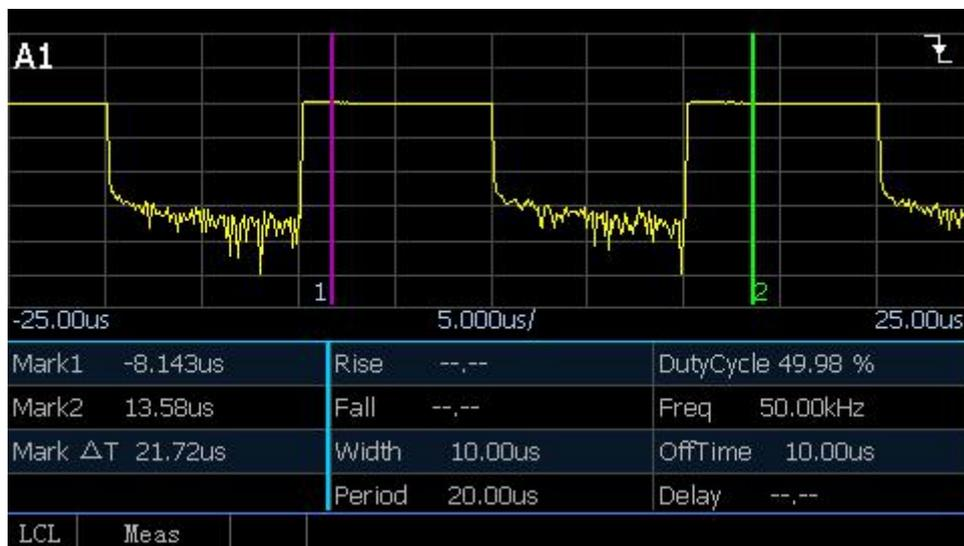
Fig. 3.3 Automatic measurement of time parameters in several periods
