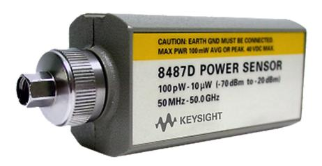
The 8487D diode power sensor measures average power over the frequency range 50 MHz to 50 GHz and power range -70 to -20 dBm (50 dB dynamic range)
