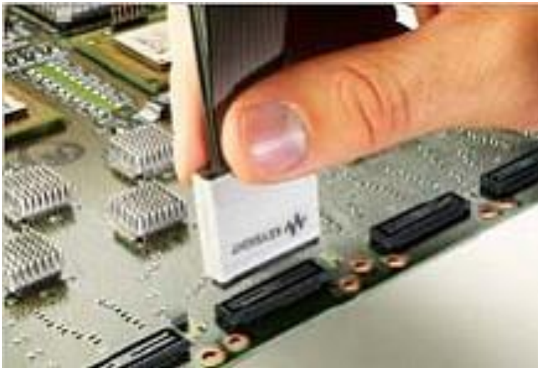
E5385A 34-channel Samtec connector probe
