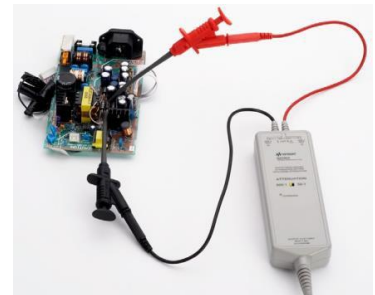
N2790A measuring a power supply signal
