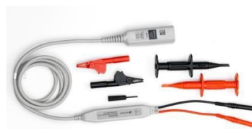
N2818A 200-MHz, 20-V differential probe
