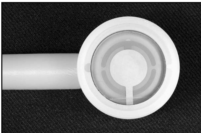
Figure 9. Crystal in place with correct electrode orientation.
