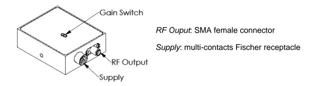
Connect the *RF Output* to a 50  $\Omega$  coupled measurement tool (e.g. oscilloscope, RF-spectrum analyzer, ...) via SMA cable.
