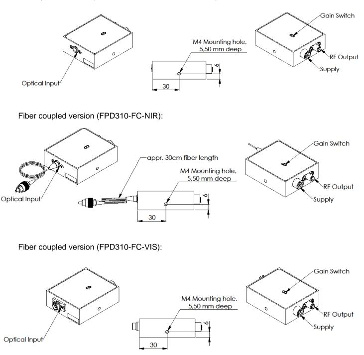
Dimensional unit is millimeter [mm].
