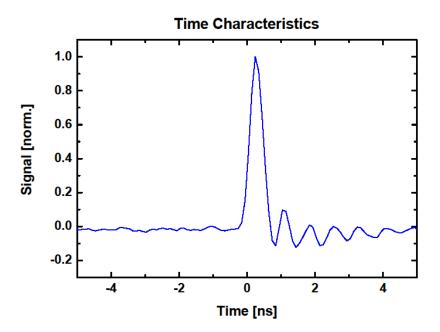
The rise time of the photodetector is defined as the time for the signal to rise from 10% up to 90% of the maximum value.
