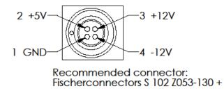
Four pole male connector on detector.
