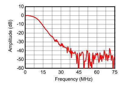
Figure 5: INT-POL-1300 MONITOR output frequency response
