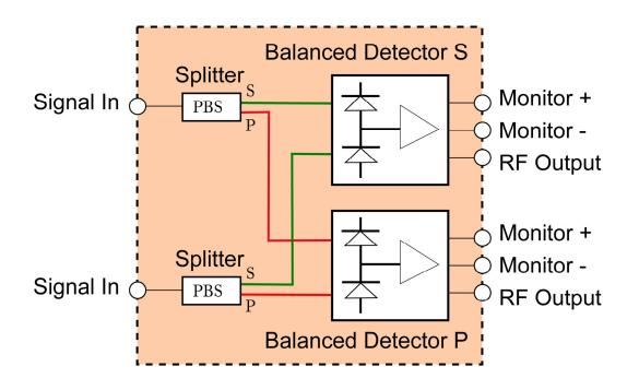
Figure 2: Functional block diagram of the INT-POL-1300
