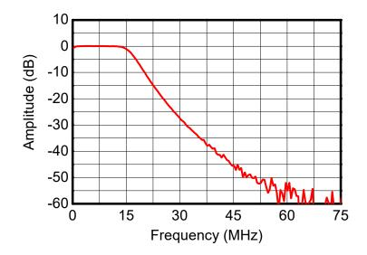
Figure 4: INT-POL-1300 RF OUTPUT frequency response
