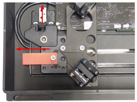
4. Push the platform to the left stop, turn the lock counterclockwise and tighten the lock screw.
