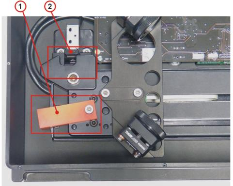
1 - Transportation Lock 2 - Electromagnetic Endpoint Latch
