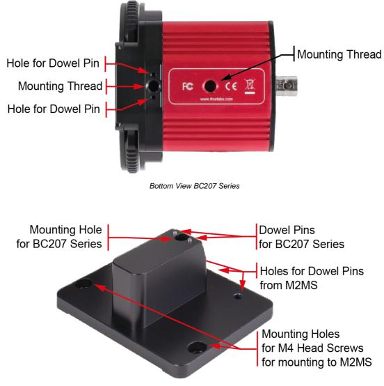
M2MS Adapter for BC207UV(/M) and BC207VIS(/M)
