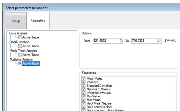
Options: Select the wavelength range. By default, the entire operating wavelength range of the recognized CCS spectrometer is stated.
