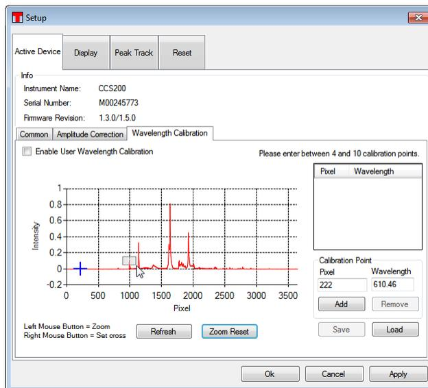
When release the left mouse button, the display appears zoomed. Move the mouse to the peak and press right mouse button. The peak will be marked now by a blue cross and the related pixel number will be displayed in the Calibration Point box:
