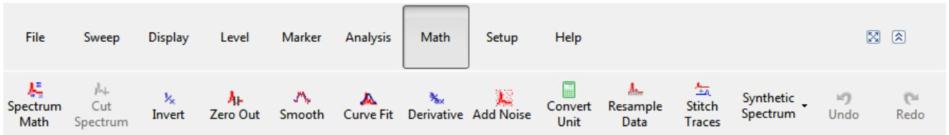
The buttons on the math menu all work on the currently active trace and are disabled while collecting spectra. The math operations can be undone by pressing the “Undo” button.
