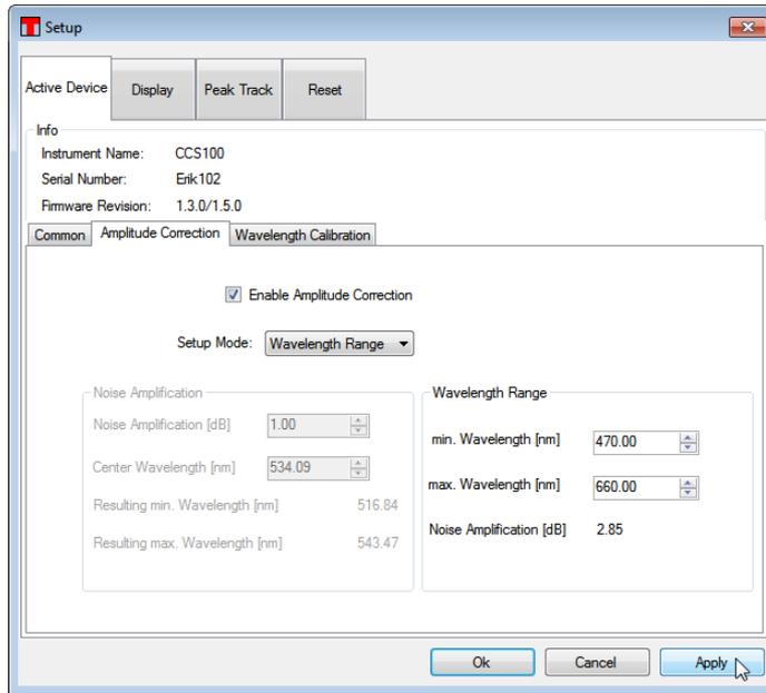
Enter the desired wavelength range; the OSA software calculates the "Noise amplification" and displays it. The screenshots below illustrate how enabling the amplitude correction affects the spectrum display of a.m. cold white LED with above settings. For better visualization, [line markers](#) are inserted at the lower and upper limit of the corrected wavelength range:
