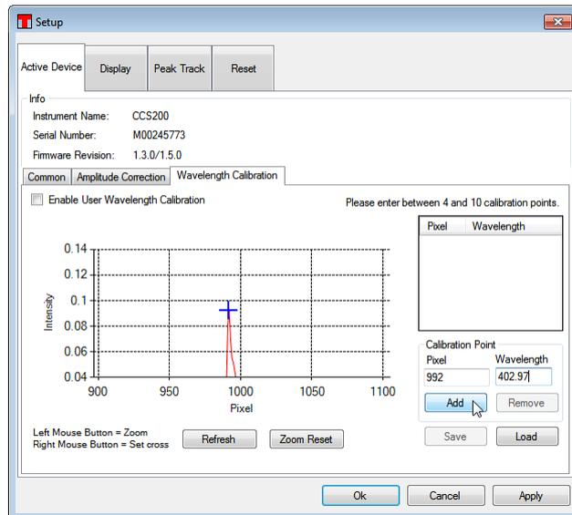
Enter the corresponding wavelength and press **Add** button - the calibration point will be added to the table. Repeat these operations until at least 4 calibrations points are entered.
