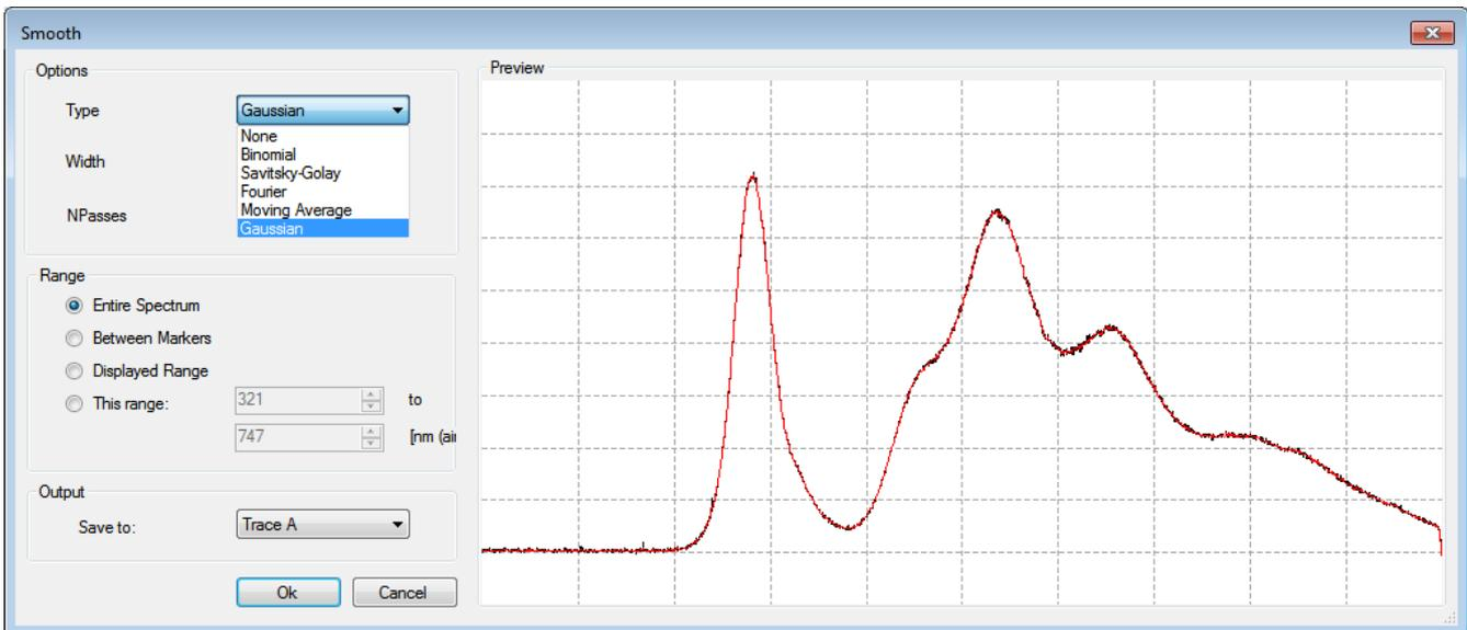
The trace to operate on is displayed in black in this dialog and the smoothed spectrum is displayed in red. Beside the displayed by default Gaussian smoothing, there are available a number of alternative smoothing methods.
