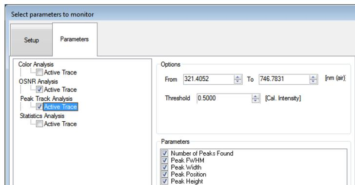
Options: Select the wavelength range. By default, the entire operating wavelength range of the recognized CCS spectrometer is stated.
