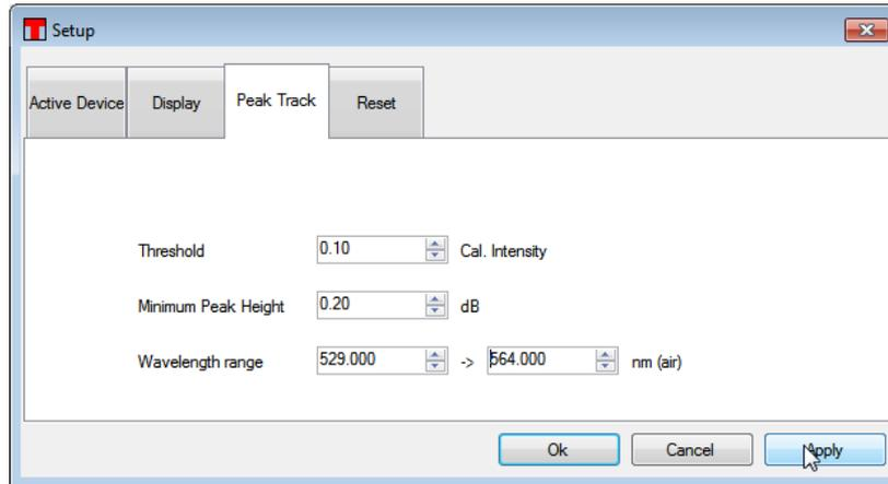
Set in the **Peak Track** tab the criteria for detecting a peak:
