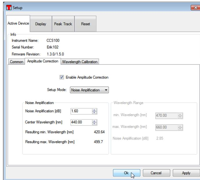
Enter the desired center wavelength and the allowed noise amplification; the OSA software calculates the resulting min. and max. wavelengths. The screenshots below illustrate how enabling the amplitude correction affects the spectrum display of a.m. cold white LED with above settings. For better visualization, a [line marker](#) is inserted at the center wavelength range:
