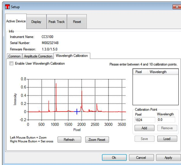
The small display can be easily zoomed by dragging the desired zoom area with left mouse button hold pressed.
