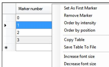
Click to a marker table element, the marked line will be highlighted and an ► appears to the left of the marked line. Right click to the table and an options menu comes up:
