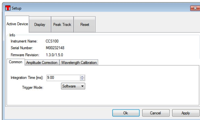
The active device tab shows information on the active instrument and has 3 sub-tabs.
