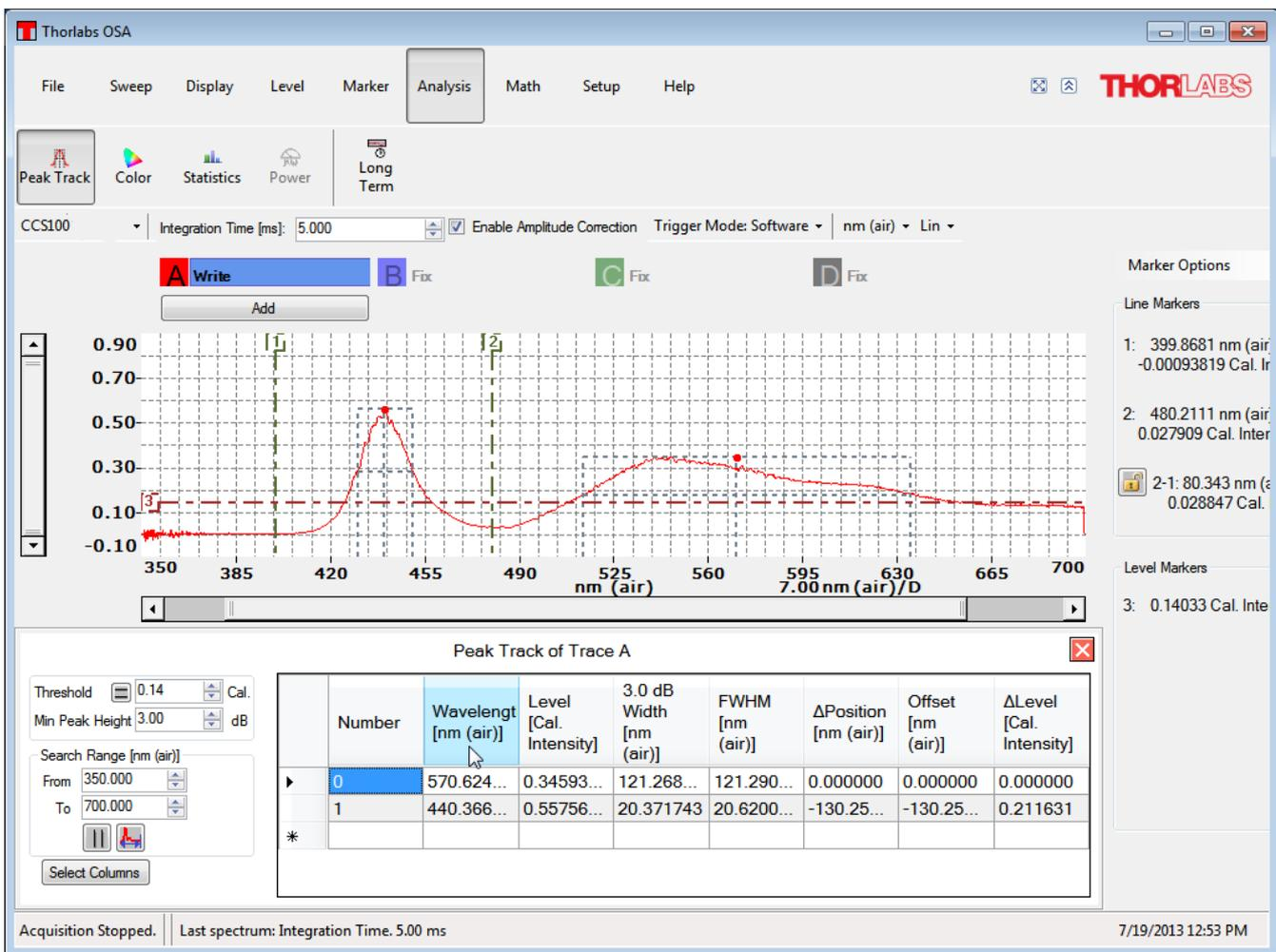
In **Peak Track** analysis mode, the position, amplitude, and width of peaks in the spectrum can be tracked over time.
