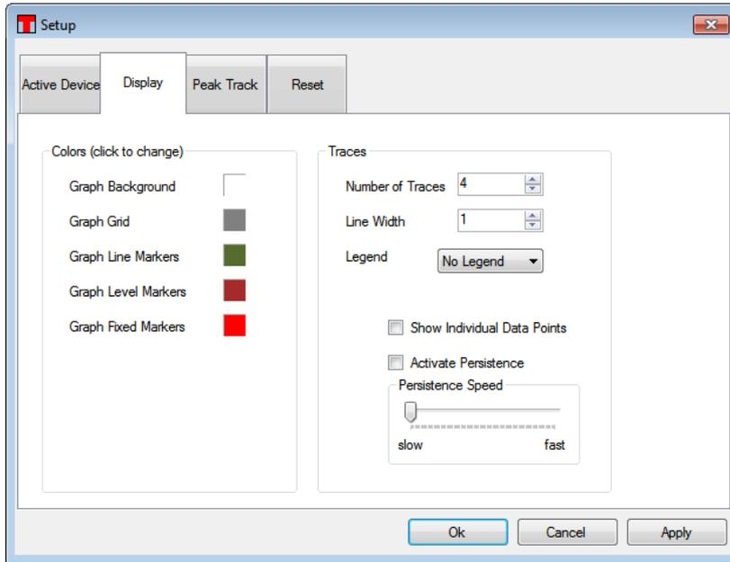
The left part is dedicated to the color setup of the graphic elements in the spectrum display. Click to a color to open the Windows color setup dialog. In the right part, the common settings of the [traces](#) can be configured:
