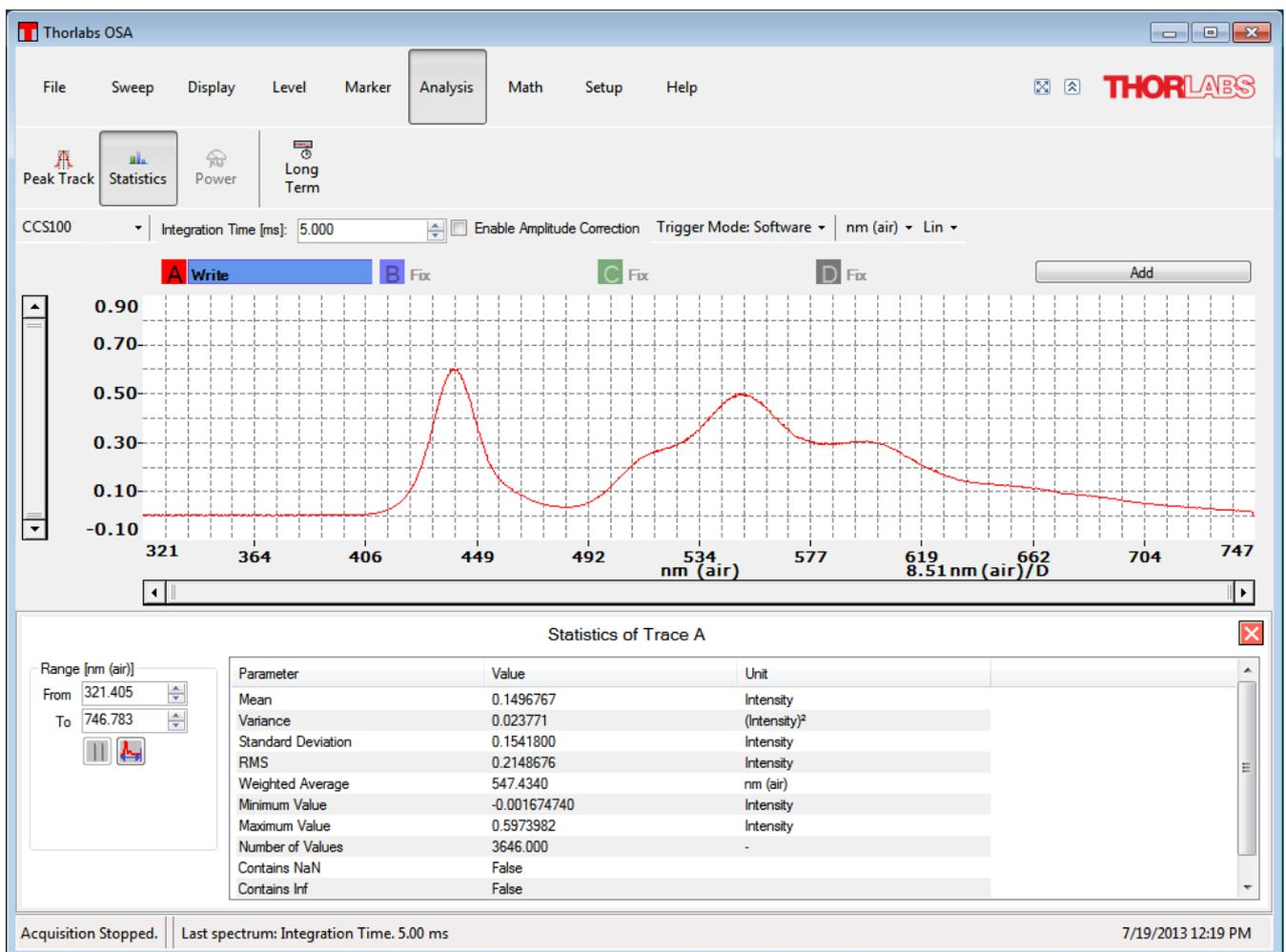
The **Statistics** function displays statistical values of the acquired spectral intensities over the specified wavelength range.
