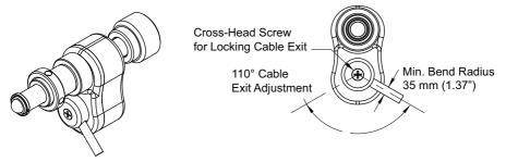
Fig. 3.1 Adjusting the Cable Exit Position
