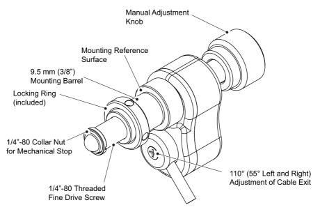
Fig. 2.1 PIA Series Piezo Inertia Actuator - Features
