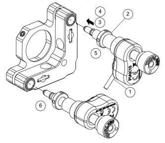
Fig. 3.3 Fitting the PIA10K to a KM100 Mirror Mount
