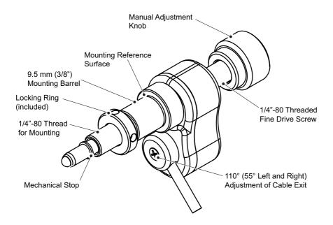
Fig. 2.2 PIAK10 Piezo Inertia Actuator - Features
