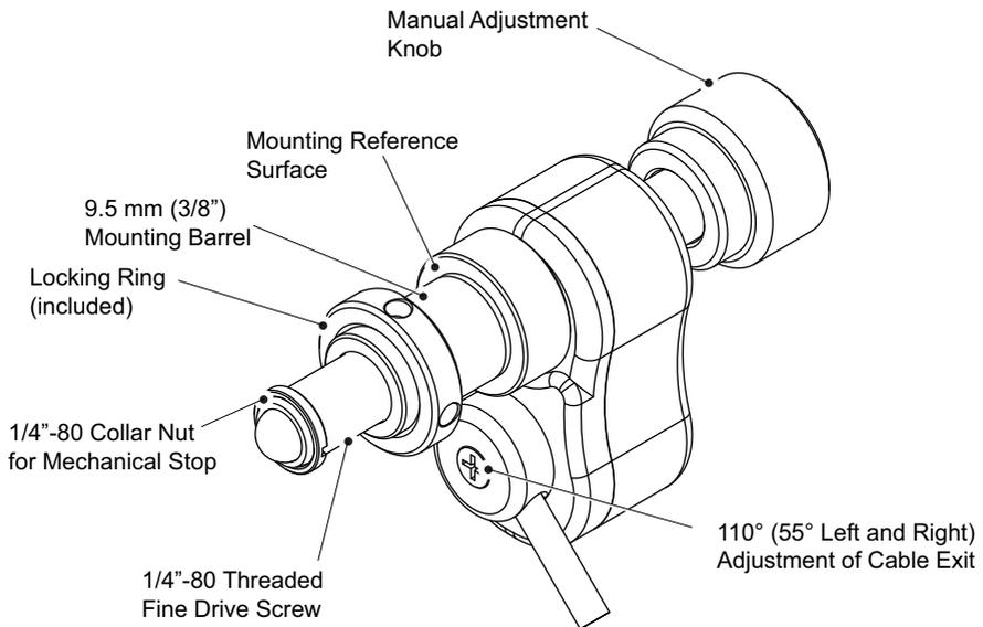
**Fig. 2.1 PIA Series Piezo Inertia Actuator - Features**
