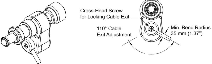
Fig. 3.1 Adjusting the Cable Exit Position
