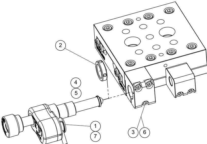
Fig. 3.2 Fitting a PIA25 to a LNR25 Stage
