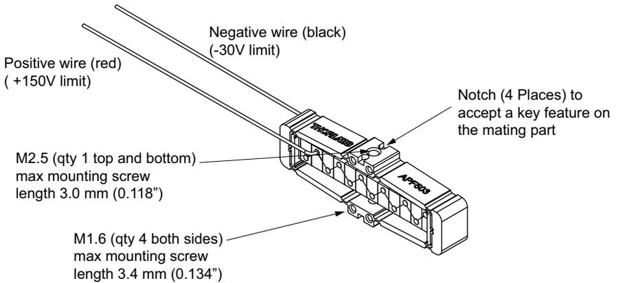
**Fig. 3.2 Fitting the APF5 series piezo actuator**
