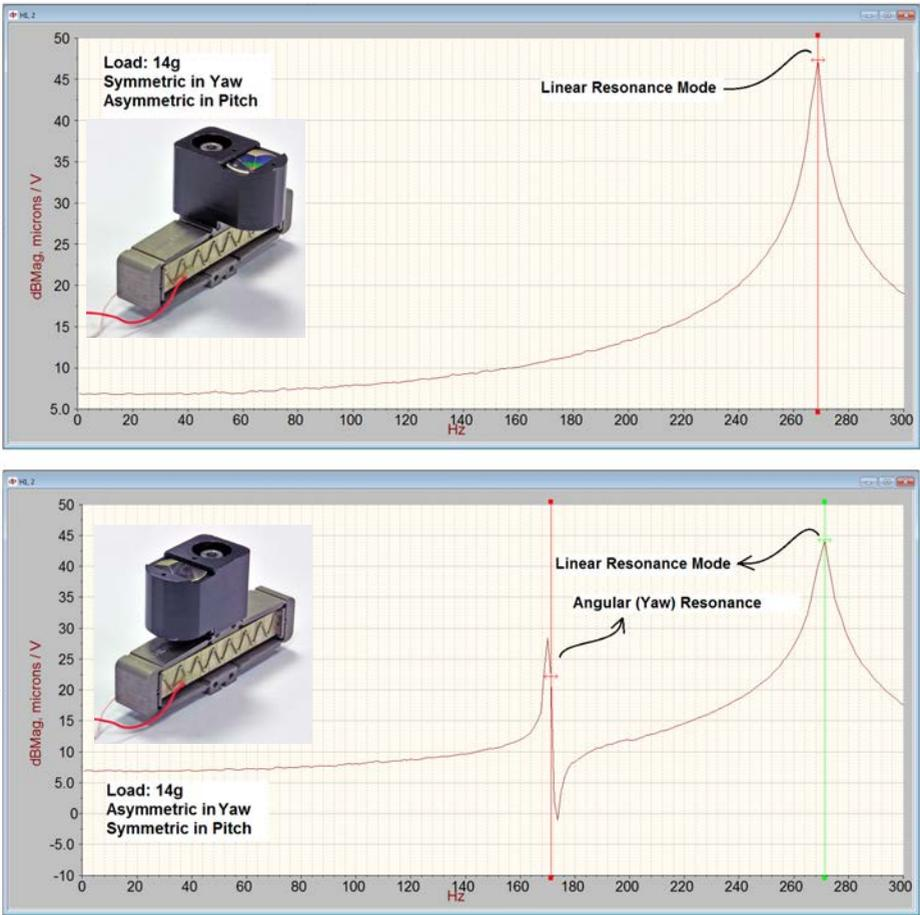
Fig. 5.1 Effect of assymmetric loading on resonance mode, linear v angular
