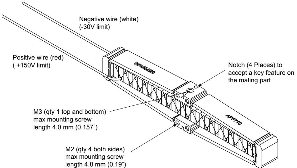
Fig. 3.1 Fitting the APF7 series piezo actuator
