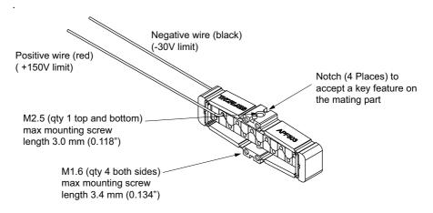
Fig. 3.2 Fitting the APF5 series piezo actuator
