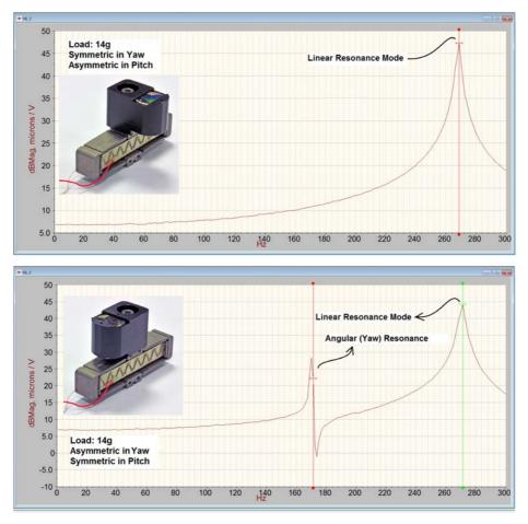
Fig. 5.1 Effect of assymetric loading on resonance mode, linear v angular
