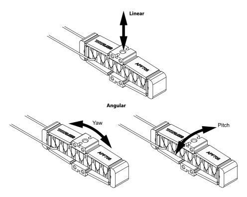
Fig. 5.2 Definition of linear and angular resonance modes
