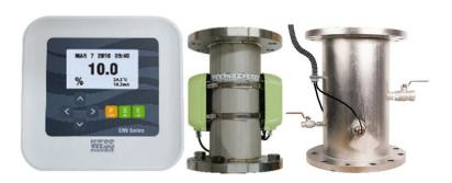
The ENV200 is an ultrasonic instrument that measures the density of suspended solid in liquid. The ENV200 utilizes the EEA (Envelope Energy Average) method that saves reception signal envelop and then calculates its energy, rather than using the reception signal's amplitude change. ENV200 comprises of a controller and two types of sensors, such as Spoolpiece and Clamp-on type to accommodate all field demands at installation.
