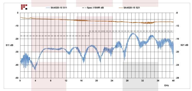
10 dB Fixed Attenuator 2.92mm Male To 2.92mm Female Directional Up To 40 GHz Rated To 10 Watts With Passivated Stainless Steel Body from Fairview Microwave is in-stock and available to ship same-day. All of our RF/microwave products are available off-the-shelf from our ISO 9001:2008 certified facilities in Allen, Texas. Fairview Microwave is RF on-demand.
