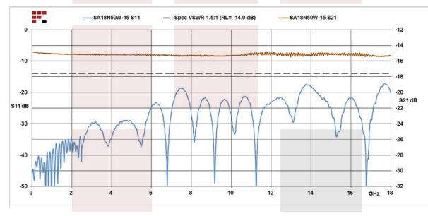
15 dB Fixed Attenuator N Male To N Female Up To 18 GHz Rated To 50 Watts With Black Aluminum Heatsink Body from Fairview Microwave is in-stock and available to ship same-day. All of our RF/microwave products are available off-the-shelf from our ISO 9001:2008 certified facilities in Allen, Texas. Fairview Microwave is RF on-demand.
