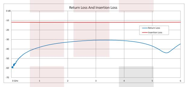
12 dB Fixed Attenuator SMA Male To SMA Female From 0.009 MHz To 6 GHz Rated To 2 Watts With Brass Body from Fairview Microwave is in-stock and available to ship same-day. All of our RF/microwave products are available off-the-shelf from our ISO 9001:2008 certified facilities in Allen, Texas. Fairview Microwave is RF on-demand.
